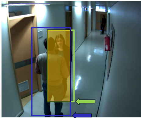
Fig. 4. Example of two overlapping detections and determination of which is occluded. The two Bounding Boxes have a high degree of overlap as shown by the yellow area in the image. In a pair of overlapping detections the one with a higher positioning of its Bounding Box lower boundary (see the arrows) is the occluded one based on geometric considerations. Thus in this image, the woman is heavily occluded.
